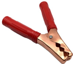
735-0155 41A COPPER 200 AMP CLAMP UP TO 1 AWG RED (6"OAL)
