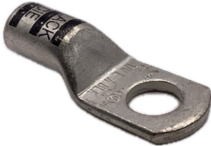
737-0358 1/0 AWG 1/2 HOLE HEAVY DUTY COPPER LUG TIN PLATED
