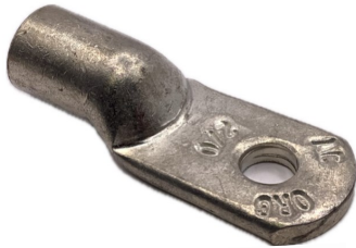
737-0365 2/0 AWG 5/16 HOLE HEAVY DUTY COPPER LUG TIN PLATED
