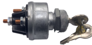
31-610 4 POSITION ACC-OFF-ON/ACC-START SPRING RETURNS TO ON 5 STUD TERMINALS
