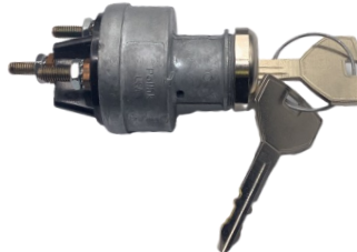
31-242 4 POSITION ACC-OFF-ON/ACC-START SPRING RETURNS TO ON 5 SCREW TERMINALS
