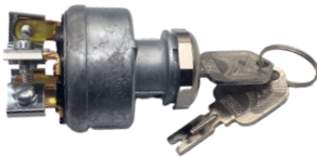
31-242 4 POSITION ACC-OFF-ON/ACC-START SPRING RETURNS TO ON 5 SCREW TERMINALS
