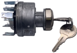
31-114 4 POSITION ACC-OFF-ON/ACC-START SPRING RETURNS TO ON 11 BLADE TERMINALS HOUSING TIED TO GROUND TERMINAL
