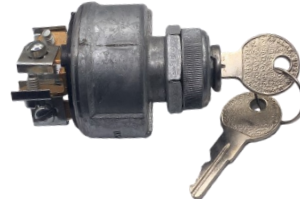
31-105 4 POSITION ACC-OFF-ON/ACC-START SPRING RETURNS TO ON 5 STUD TERMINALS
