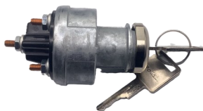
31-527 4 POSITION ACC-OFF-ON/ACC-START 4 STUD TERMINALS DESIGNED W/GLOW PLUG "WARM" POSITION
