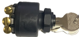
33-105 3 POSITON OFF-ON/ACC-START SPRING RETUNS TO ON "PUSH TO CHOKE" FEATURE MAGNETO GROUNDED 6 SCREW TERMINALS MARINE
