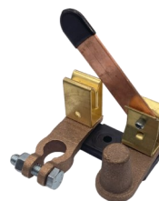
854-0138 5/8" DIAMETER POST FOR RECEIVING STANDARD BATTERY CLAMP MOUNT ON NEGATIVE BATTERY POST TO DISCONNECT GROUND AND BATTERY
