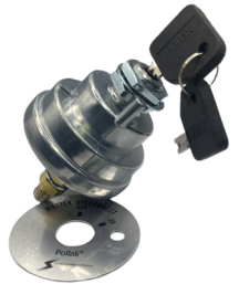
51-316 SPST 2 POSITION OFF-ON 6-36V 2 STUD TERMINALS 2 REMOVABLE KEYS
