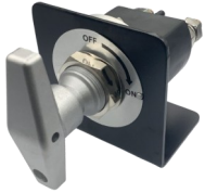
854-0247 RATED 500 AMP CONTINUOUS 5000 AMP SURGE @ 12V WATER RESISTANT
