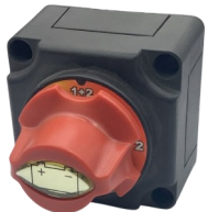
854-0387 2 POSITION CRANK RATING 700 AMP/10 SECONDS CONTINUOUS RATING 300 AMP INTERMITTENT RATING 1000 AMP/5 SECONDS APPLICATION UP TO 48V
