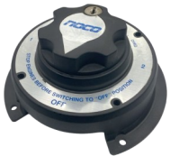
854-0360 4 POSITION BOTH/1/2/OFF 6-36V CONTINUOUS RATING 310 AMP INTERMITTENT RATING 500 AMP FOR 5 SECONDS DISCONNECT/SELECTOR SWITCH
