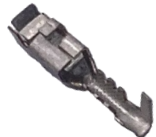
844-20230 22-20 AWG CABLE DIAMETER RANGE 1.3MM TO 2.19MM FUEL INJECTOR TERMINAL
