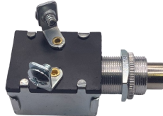
24-360 SPST 2 POSITION OFF-MOM ON 60 AMP @ 12V 2 STUD TERMINALS WEATHER/DUSTPROOF
