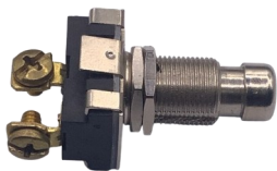
30-1426 SPST 2 POSITION OFF-MOM ON 15A @ 12V 2 SCREW TERMINALS
