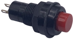
24-350 SPST 2 POSITION OFF-MOM ON 3 AMP @ 12V 2 SOLDER TERMINALS MINIATURE SIZE
