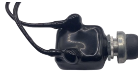
24-372 SPST 2 POSITION OFF-MOM ON 70 AMP @ 14V 2 BLADE/SCREW COMBO TERMINALS BRASS/CHROME PROTECTIVE COLLAR
