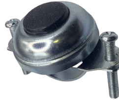
52-777 SPST 2 POSITION OFF-MOM ON 2 SCREW TERMINALS
