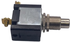
24-355 SPST 2 POSITION OFF-MOM ON 15 AMP @ 12V 2 SCREW TERMINALS
