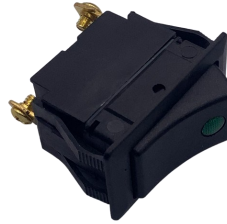
34-306 SPST 2 POSITION ON-OFF 20 AMP @ 12V 3 SCREW TERMINALS GREEN PILOT LIGHT
