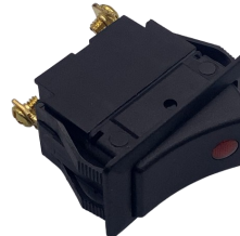
34-230L SPST 2 POSITION ON-OFF 20 AMP @ 12V 2 BLADE TERMINALS LED PILOT LIGHT
