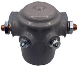
52-315 100 AMP @ 12V CONTINUOUS DUTY INSULATED DUST & MOISTURE RESISTANT
