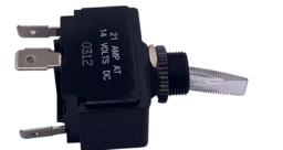
34-586 SPST 2 POSITION ON-OFF 20 AMP @ 12V 4 BLADE TERMINALS LIGHTED HANDLE
