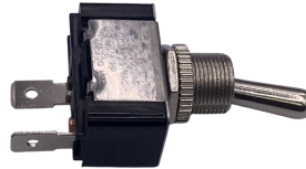
34-570QP SPST 2 POSITION MOM ON-OFF 20 AMP @ 12V 2 BLADE TERMINALS
