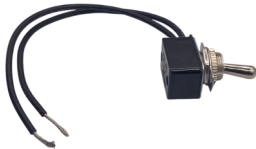
34-513 SPST 2 POSITION ON-OFF 10 AMP @ 12V 2 18 AWG WIRE LEADS
