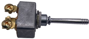
34-220 SPDT 3 POSITION MOM ON-OFF-MOM ON 50 AMP 6-24V 3 SCREW TERMINALS 1-1/2" LONG HANDLE
