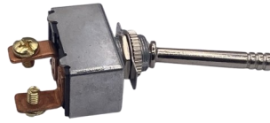
34-213 SPST 2 POSITION ON-OFF 50 AMP 6-24V 2 SCREW TERMINALS 1-1/2" LONG HANDLE
