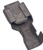
842-18690 TWO GAUGE LEADS: 16-14 AWG OR ONE GAUGE: 12 AWG FITS 5/16" MALE TAB
