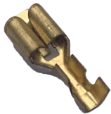
838-14892 GM, FORD, CHRYSLER UNIVERSAL TERMINAL 20-18 AWG 1/4" FEMALE
